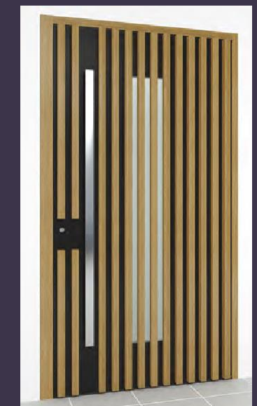
Model 466 Glazed 3D door design with 40mm x 40mm box sections bonded onto the outside of the door sash (Glass can be clear, full satin or satin with clear lines).
